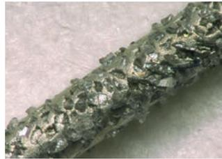
A large number of diamond wires offered by Diamond WireTec are produced in-house. The diamond wires differ in the type of diamond bonding, the diamond density, the wire diameter and the strength. These are important properties for a clean and economical separation cut.
