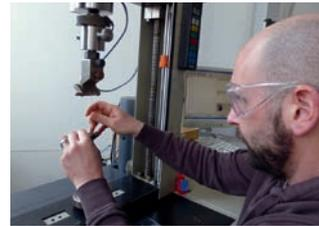
All diamond wires offered by Diamond WireTec are subject to a 100% check and the strictest requirements. Tension tests for examining the stretching properties and strength as well as microscopic visual tests for the overall assessment are part of our quality management system.
